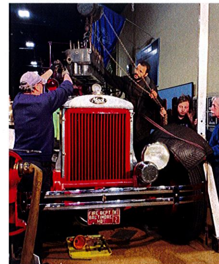
2022-3-29, Hale-Mack water tower, hoisting cylinder block, T Miller, D Shimp, A Krongard, S Heaver
